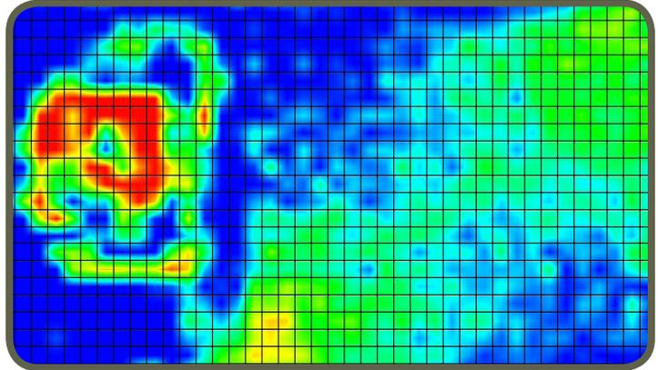
During any new PCB development process, design engineers must find, characterize, and address unintended radiators or RF leakage to pass compliance testing. EHX allows board designers to pre-test and resolve EMC and EMI problems early on, thus avoiding unexpected EMC compliance test results.
