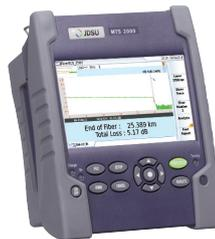
One-Slot Handheld Modular Platform Singlemode/Multimode Fiber Testing
